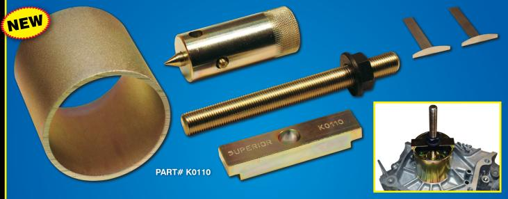
The K0110 Kit is designed to safely and easily remove the secondary shaft bearing and oil collar without damaging the bearing, collar or bell housing. If you work on Honda or Acura transmissions, this is a must have tool for your workstation or toolbox. With the Superior Transmission Parts, Inc. K0110 Honda/Acura Large Collar Puller Kit you can remove the bearing and collar in just under 5 minutes!
