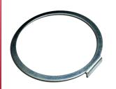
Our K0126 Dodge O.D. bearing support shim is the Superior Solution® to saving worn support / tail housings on most late model 42 / 46 / 47 & 48RE transmissions. It takes up excessive clearance and features a lock tab "no-spin" design to prevent further wear. Shim it up and "Keep it Tight - Do it Right!"
