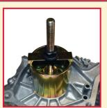
The Honda/Acura Small (K0135) & Large (K0110) Collar Puller Kits are designed to safely and easily remove the secondary shaft bearing and oil collar without damaging the bearing, collar or bell housing. With these kits, you can remove the bearing and collar in just under 5 minutes!
